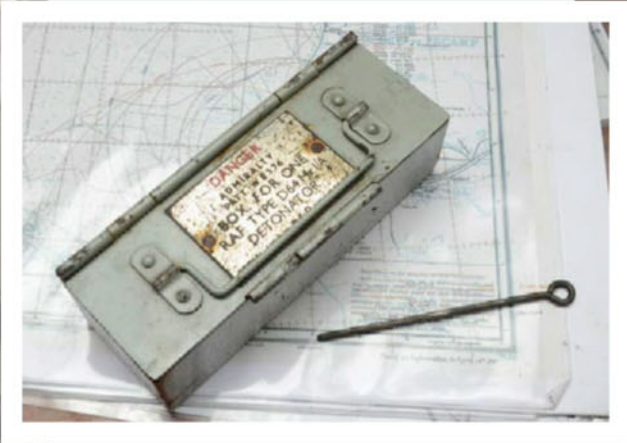
This box (left) contained a detonator that was to be used by the commanding officer to destroy all the classified equipment on the vessel, if it were at risk of being captured by the enemy
